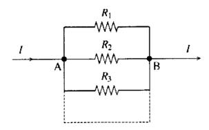
For resistors connected **in parallel** the voltage is the same for all individual resistors because they are all connected to the same two points (A and B on the diagram). The total current is the sum of the currents through the individual resistors. This should makes sense as the total current "splits" at points A and B.
