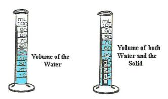
**Volume determined by water displacement**. The change in volume is equal to the volume of the solid.
