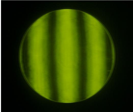
**Ronchi test image of 10-inch telescope mirror that has been in storage in the Geoscience Department.**
