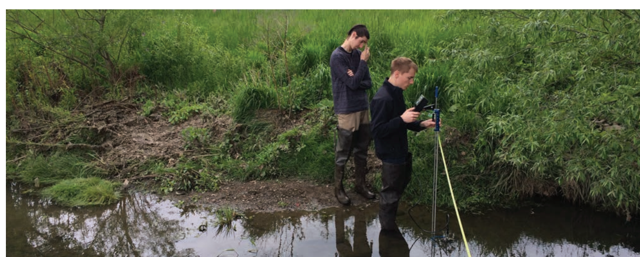
Students are also in the process of creating Stage-Discharge rating curves to allow for the calculation of estimated discharge on many of these streams.
