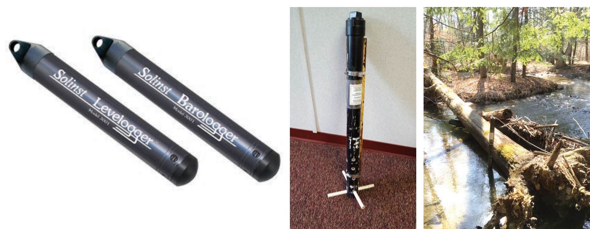
Left: Solinst Levelogger and barologger, Middle: PVC pipe installation setup, Right: Lauren Run data logger location
