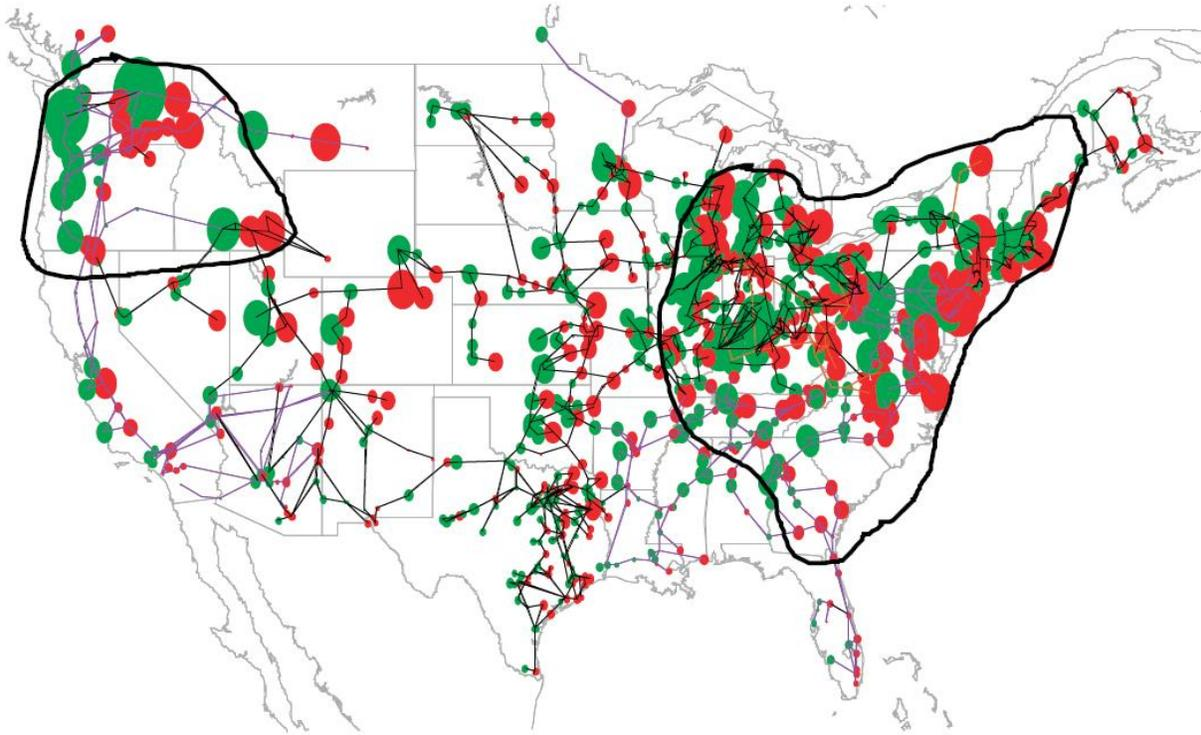
Scenario showing effects of a 4800 nT/min geomagnetic field disturbance at 50° geomagnetic latitude scenario. The regions outlined are susceptible to system collapse due to the effects of the GIC disturbance; the impacts would be of unprecedented scale and involve populations in excess of 130 million. SOURCE: J. Kappenman, Metatech Corp., "The Future: Solutions or Vulnerabilities?," presentation to the space weather workshop, May 23, 2008.
