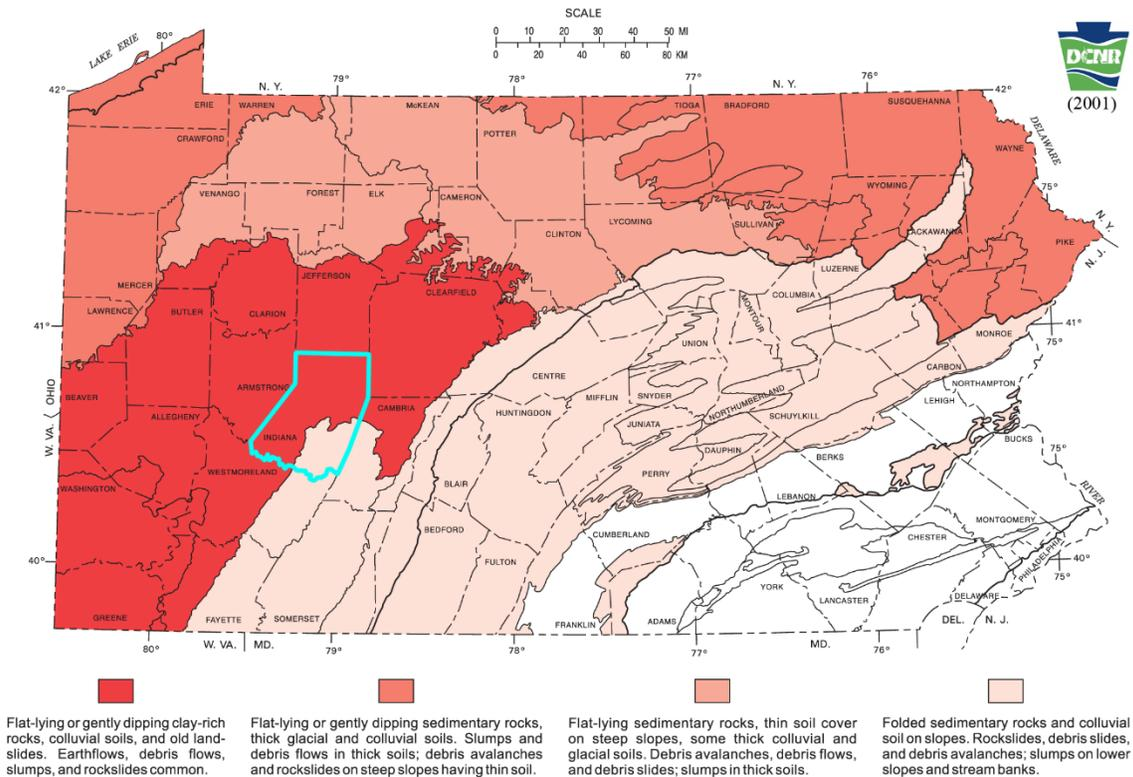
**The distribution of types of landslides most likely to occur in different geologic settings in Pennsylvania. Stream-bank slumps, soil creep, and rockfall/rockslide combinations on cut slopes can occur throughout Pennsylvania.**
