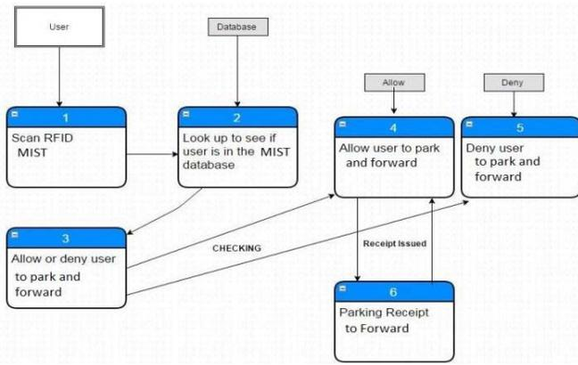
Fig. 2. High-level system prototype schematic.
