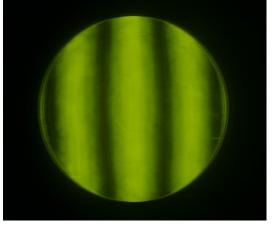
Ronchi test image of 10-inch telescope mirror that has been in storage in the Geoscience Department.
