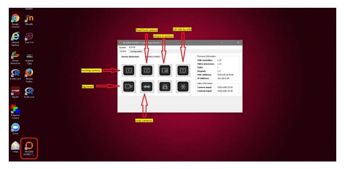
The two cameras are noted and pressing either "1" or "2", will only provide that camera as the source. As noted in the screenshot, there are three ways to combine both cameras into one video source. There is "picture in picture", "full side by side" and big/small. The "swap cameras" button reverses the position of the cameras in the layout. This app can be minimized once you set it up.
